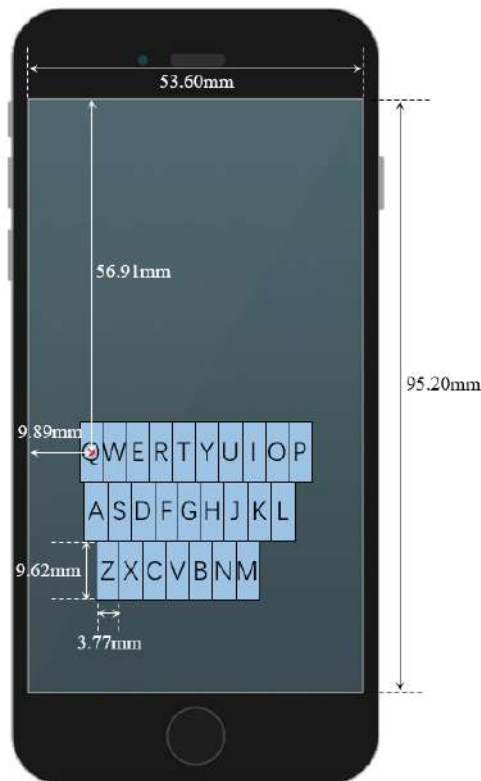
Fig. 6. The general user keyboard (in absolute model) fitted from pooled data of the 12 users in Study 1. The red dot represents the centroid of the key 'Q'.
