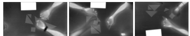
Figure 4: Tabletop workspace with (left) two forearm leans framing a closed personal space, (center) right user creating an open space with forearm and elbow, and (right) two forearm lean contacts forming a partially open personal space. Bright regions are paper sheets presenting the task; such shapes are not yet recognized by our method.
