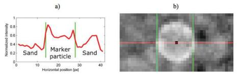
Fig. 7. An intensity profile (a) obtained along the red line, as shown in (b).
