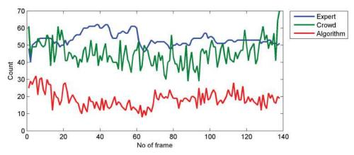
Fig. 12. The number of particles detected in each frame of the sample by the expert (blue), the crowd (green) and the algorithm (red) for the 6-dense-B dataset.
