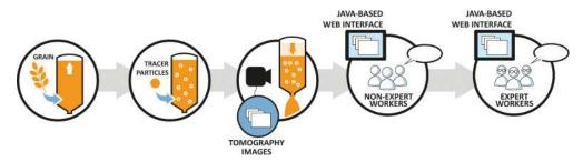
Fig. 1. Overall workflow, from left to right: Silo is filled with material mixed with tracer particles. Tomographic images are taken of the silo flow as it is emptied, images are sent to the web interface for analysis by nonexpert workers, then expert workers verify the analysis.
