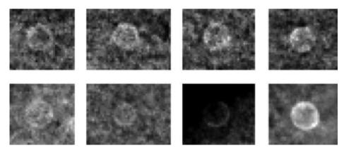
Fig. 6. Typical shapes of particles that can be found in the loose flow (top row) and dense flow (bottom row) datasets. The images were obtained during flow experiments. Images are enlarged with no pixel approximation method (or nearest neighbor). Note the low SNR of the images, which effectively limits the variety of applicable detection algorithms.
