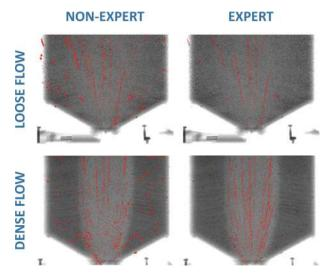
Fig. 9. Results from experiment comparing accuracy of trajectories between expert and nonexpert workers for both loose and dense flows, without eliminating particles that are identified by only one worker.
