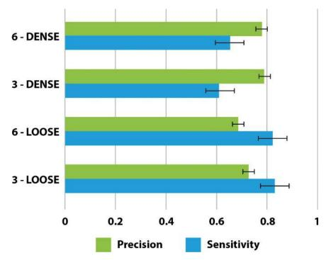
Fig. 10. Precision and sensitivity for the four experiment conditions. Note that, for the dense dataset, an increase in the number of tasks per frame yields better sensitivity, while the effect was not observed for the loose dataset. Error bars are .95 confidence intervals. The results on the graph are provided without eliminating particles that were identified by only one worker.
