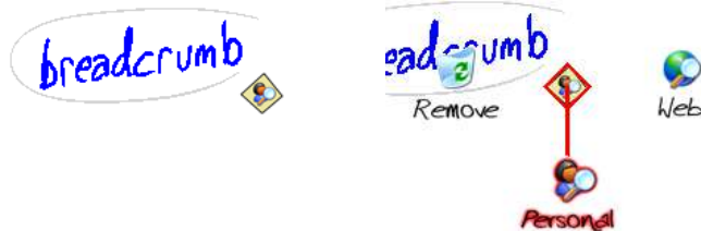
Fig. 3. Breadcrumb. Left: The user presses a button to enter gesture mode [18] and lassos some ink. The breadcrumb icon appears on pen-up. Right: The user can later stroke down to open Personal search results; on pen-up, the results appear (Fig. 1).
