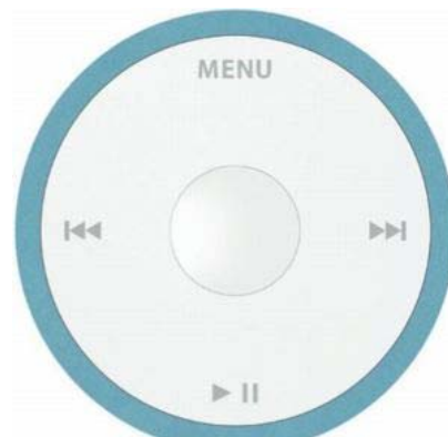
Figure 2.4: Apple's ClickWheel is a hybrid input device that combines touchpad with keypad.
