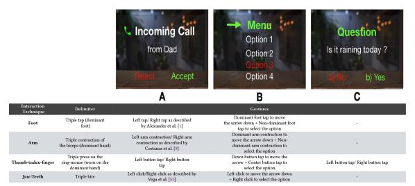
Table 1: Interactions that participants performed for the 3 different tasks (A, B, and C) that were prompted on the smart glasses. Task A (call) and Task B (menu selection) were used in both Study 1 and 2 while Task C (SMS response) was used only in Study 2.
